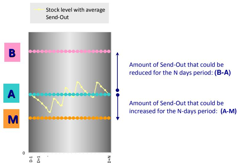
Let  $f_{\text{Send-Out}}$  be the interval showing the flexible level of Send-Out for the N-days period. It is shown,
